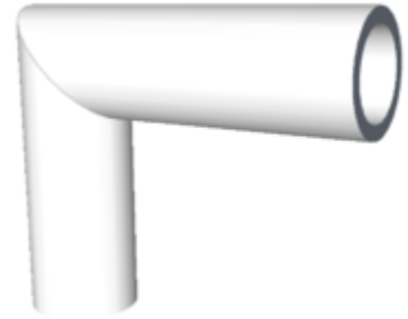
Miter joint of two pipes
