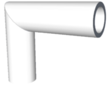
Miter joint of two pipes
